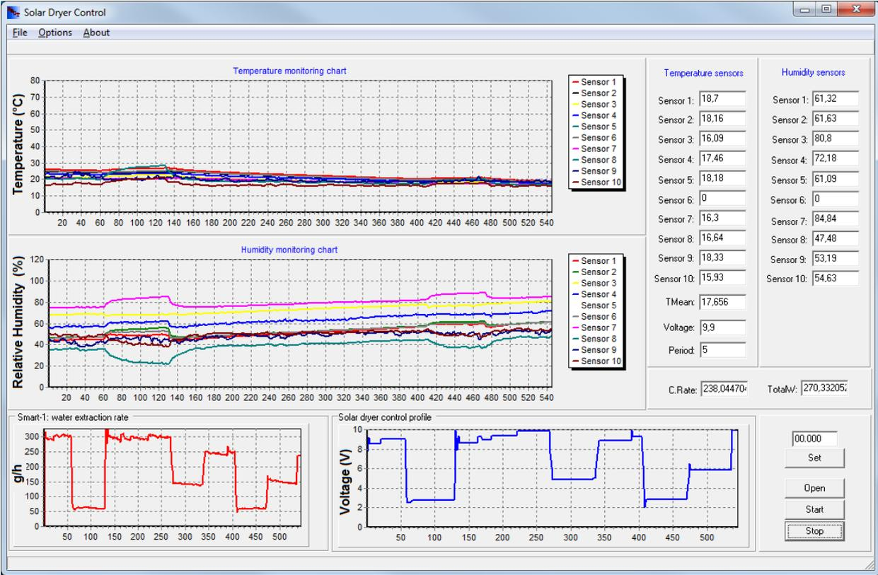
**FIGURE 2: Developed fuzzy logic control software. Temperature and relative humidity charts obtained for the optimal control profile of the solar dryer fan to achieve randomly selected water behavior profile; experimental water extraction rate SMART-1.**
